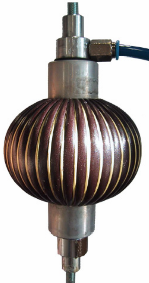
Figure 2.1: The Pleated Pneumatic Artificial Muscle
