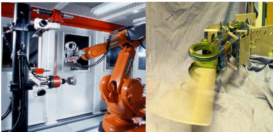
Figure 1.1: Industrial robot with heavy electrical drives and the soft actuator AMASC
